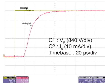
Figure 6: Typical step response (0 to 4200 V)
