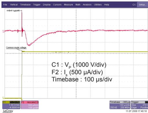
Figure 11: Typical common mode perturbation (4200 V step with 6 kV/μs,  $R_M = 100 \Omega$ )
