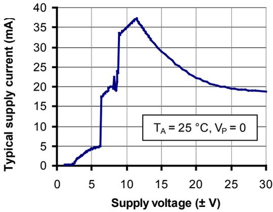
Figure 7: Supply current function of supply voltage
