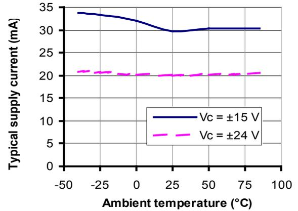
Figure 8: Supply current function of temperature
